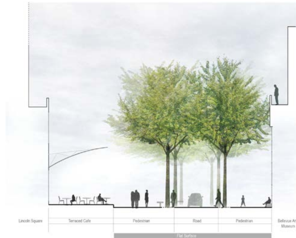
▲ Option One Recommendation for the Pedestrian Corridor - Section - Image by Balmori Associates
